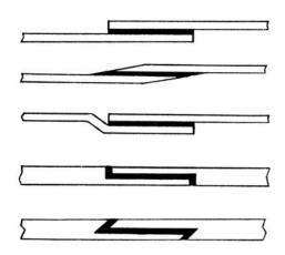
The simple lap joint is off-set when using thin materials. This can result in cleavage and peel stress under load.
